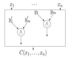
We have seen above how to approximate a single AND gate, which means that there is a polynomial  $\hat{p}$  which differs from  $y_1 \cdots y_m$  on at most  $2^m/2^r$  values. We use this result to approximate an entire circuit.
